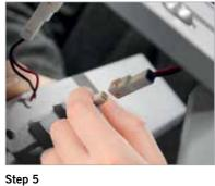
Plug in new LED chevron using existing 'plug and play' connectors on the luminaire spine
