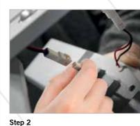
Disconnect the old LED chevron using the 'plug & play' connectors
